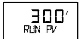
1. Run PV: Process Value - valve stroke %
