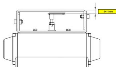
6. Attach the positioner to the bracket. Fix the clamping pin on the main shaft's center of the positioner and insert connection pin into the fork lever slot. This will lock to the fork lever spring. Setting alignment of the main shaft of the positioner and center of the actuator's stem is very important. Poor alignment of the main shaft and the actuator's stem decreases the positioner's durability due to unnecessary forces on the main shaft.
