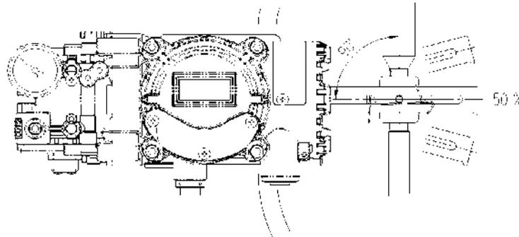
8. Check the valve stroke. The stroke marks are indicated on the feedback lever of the positioner. Position the connection pin at the number on the feedback lever which corresponds to the desired valve stroke. To adjust, move the bracket, the connection pin or both.
