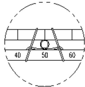
⑥ Insert connection bar into SPTM-6VL feedback lever. The connection bar should be inserted at the 50% point on the feedback lever, which would help to reduce hysteresis. <Fig 4>
